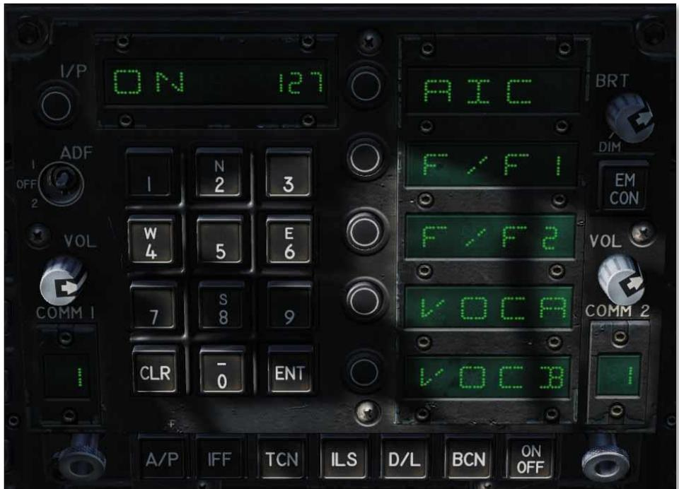
Figure 129. UFC Data Link (D/L)
